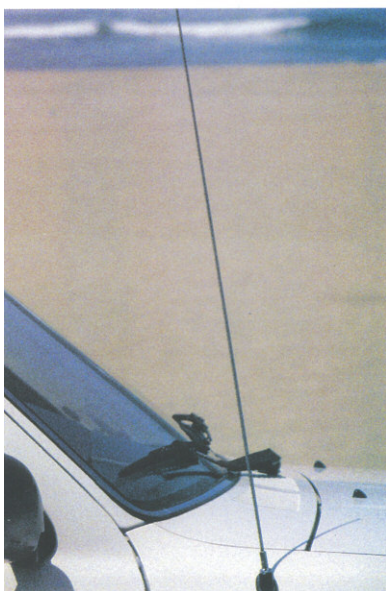
Fig. 17-11 Electrons in a radio receiving antenna respond to the electric field produced by electrons in a distant transmitting antenna.
