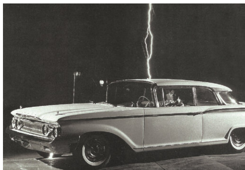
Fig. 17-25 The metal body of a car shields the interior from electric fields.
